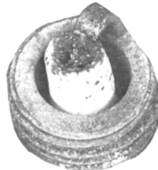
Fig. 5-19. Preignition: melted electrodes and, in most cases, a white insulator. The insulator may be discolored due to a fog of debris in the overworked cylinder. Check for correct heat range, adequate lubrication, and for overadvanced ignition timing. Correct the problem before the engine is put back into service. (Courtesy Champion Spark Plug Co.)
