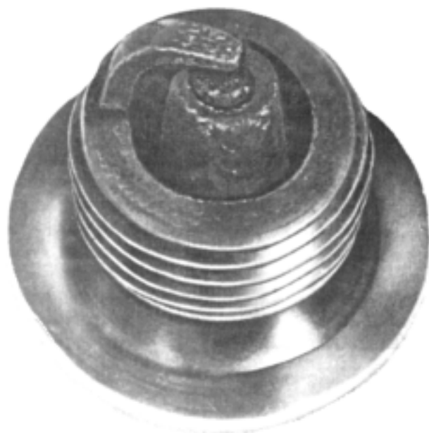
Fig. 5-11. A worn-out spark plug. (Courtesy Champion Spark Plug Co.)
