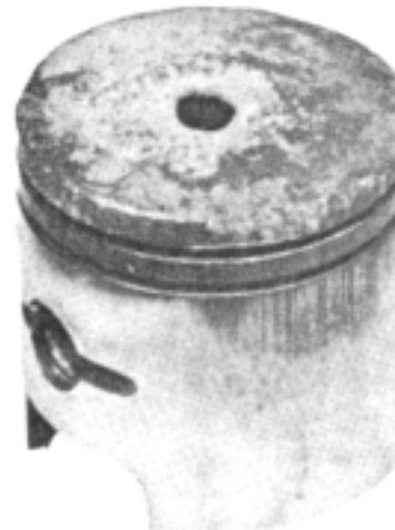
Fig. 5-8. The woeful result of pre-ignition.
