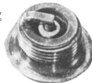
Fig. 5-15. Normal: light tan or brown, electrode wear limited to the spark zone.
