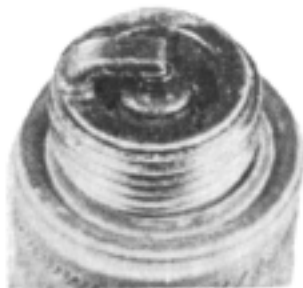
Fig. 5-17. Wet fouling: damp black carbon coating over the entire firing end. May form sludge if the condition is chronic. Check spark plug heat range (the plug may be too cold), air/fuel ratio (too rich), fuel/oil ratio (too much oil), ignition system (misfiring). (Courtesy Champion Spark Plug Co.)
