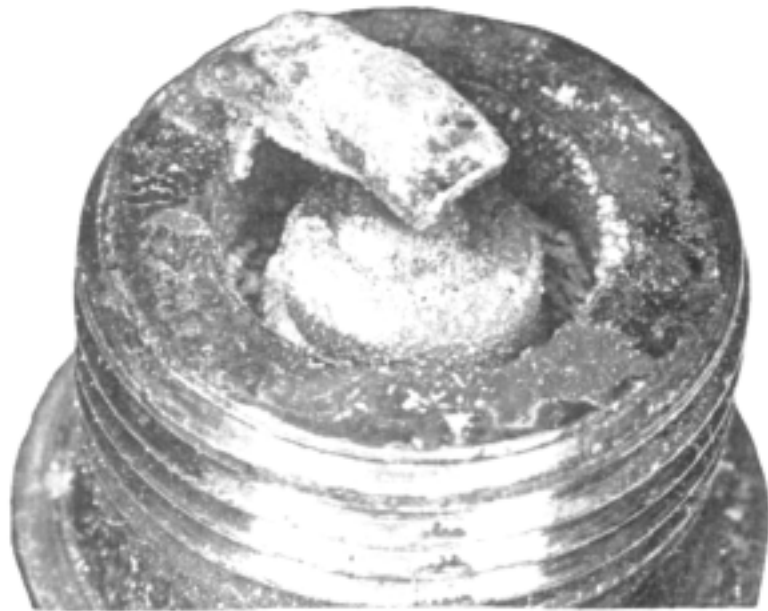
Fig. 5-20. Scavenger deposits: brown, yellow, or reddish deposits on the firing tip. These deposits are left by additives in the fuel and are not in themselves dangerous. Clean and return the plug to service. (Courtesy Champion Spark Plug Co.)
