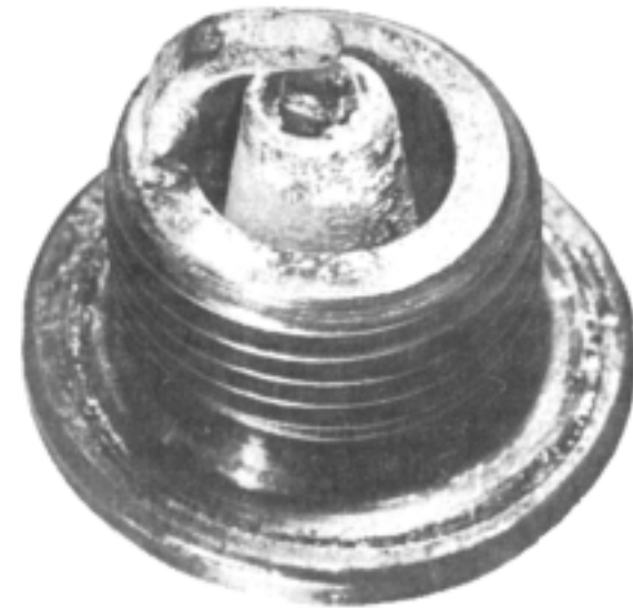
Fig. 5-18. Overheating: electrodes badly eroded, premature gap wear, gray or white insulator. Check spark plug heat range (too hot), ignition timing (too much advance), air/fuel ratio (too lean). (Courtesy Champion Spark Plug Co.)
