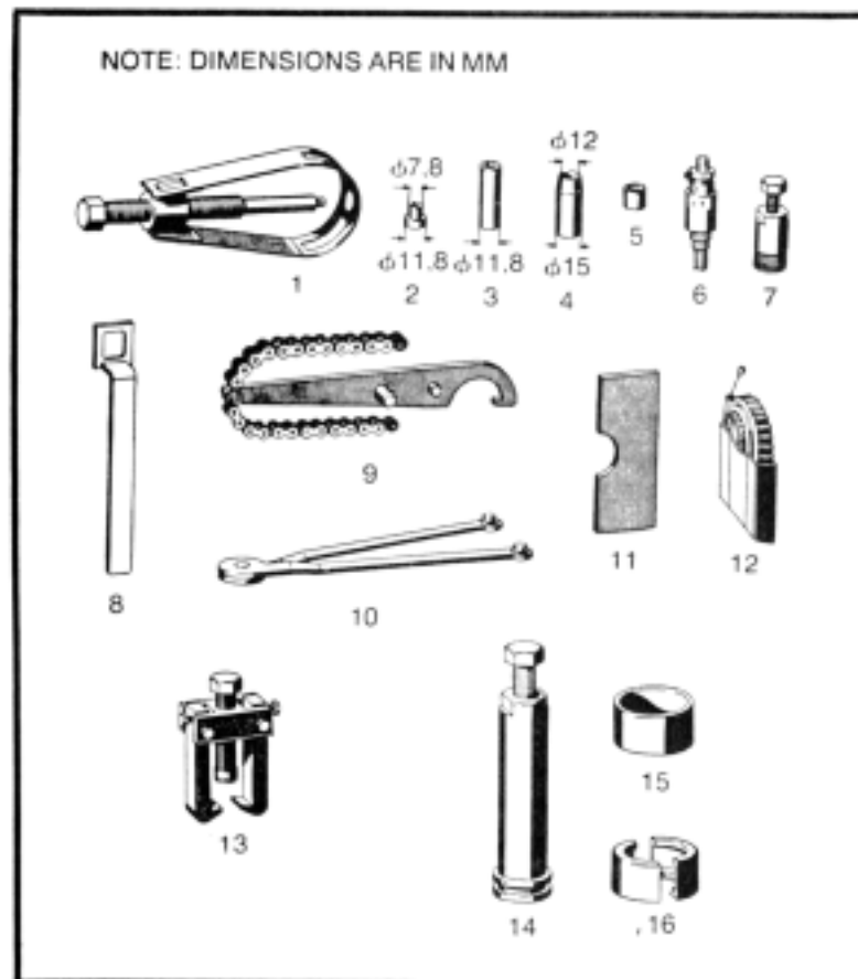
Fig. 3-17. Sachs factory tools include piston pin extractor 1, several sleeves 2, 3, 4, 5, a timing gauge 6, flywheel puller 7, offset wrench 8, clutch holder 9, flywheel holder 10, intermediate plate 11, tachometer 12, sprocket puller 13, bearing puller 14, and bearing puller adaptors 15 and 16.
