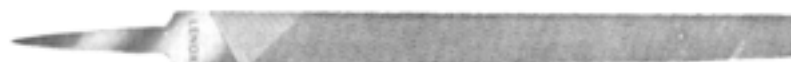
Fig. 3-13. If you buy only one file, make it a mill bastard. (Courtesy American Saw & Mfg. Co.)
