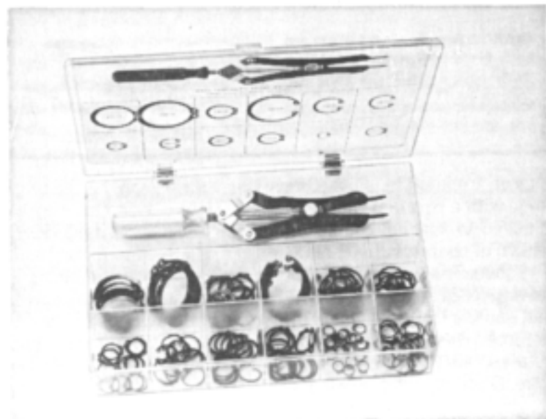
Fig. 3-12. A K-D combination snapping tool. The snapping assortment is inch standard and of no use on metric equipment.
